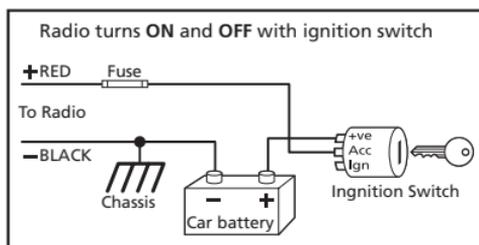
The radio should now switch ON and OFF automatically with the vehicle's ignition switch.
