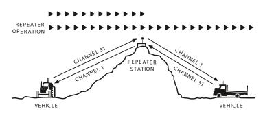
Figure 1 - Simple/Duplex Range Comparison
