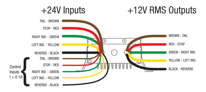
Note: VRZ(REV) features 1 single 24V power input (purple wire) rather than 4(5) individual power inputs. The VRZ(REV) still features 4(5) individual control wires and 4(5) individual RMS outputs.
