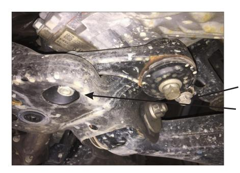
Loosen the rear mount bolts slightly. This will help with the front spacer install.
