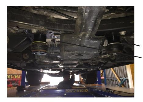
Position the 2 large mounts in position - place the part number on mounts up-wards.
