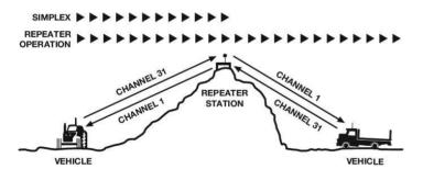
Your XRS-370C radio allows you to enable or disable Duplex mode on individual repeater channels. In this way any repeater channels that are not being used with repeaters in your area can be used in Simplex mode for normal direct radio-to-radio communications.
