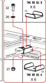
Tighten all M8 Allen cap bolts and M8 nuts using 6mm Allen key and 13mm Wrench.
