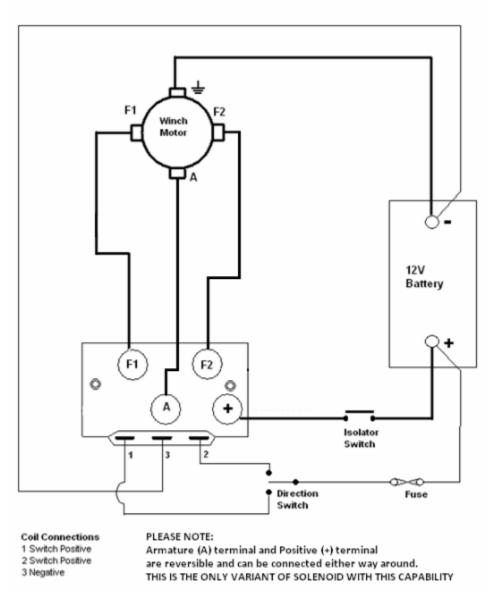
WARNING - Please ensure switch wiring on the coil is correct for rotation of motor.
