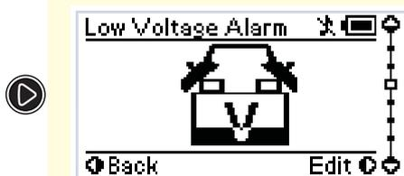
The Low Voltage Alarm setting will sound an alarm when the battery Voltage reaches a particular setting.
