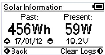
The Solar Information screen displays information on the power and voltage output of the solar panels. From this screen you can access a log of daily power generation measured in Watt Hours. The log will store up to 7 days of data and will overwrite, storing only the last 7 days at any one time.
