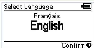
The first step required for initial setup is Language selection. Once entered the Language is set in memory and retained should power be lost and reconnected.
