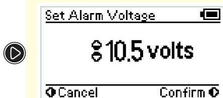
The Set Alarm Voltage setting sets the Voltage at which the alarm will sound. The Alarm Voltage can be set to OFF.
