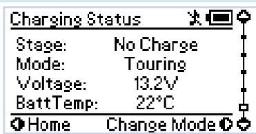
The Charging Status screen displays the charging status of The Manager30, including Charge Stage, Charge Mode and Battery Voltage and Battery Temperature.
