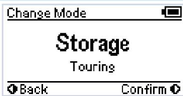
The Change Mode screen allows switching between Touring and Storage modes. Remember to disconnect all loads before setting Storage mode.
