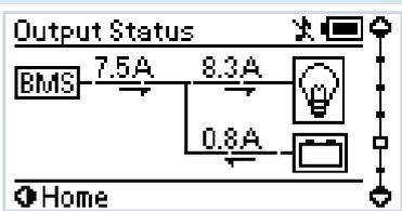
The Output Status screen displays a summary of the current flow of the system. The screen will display current from The Manager30 unit, current in to or out of the battery and current provided to the loads. The direction of the current flow is indicated by the arrows, and a moving white dot.
