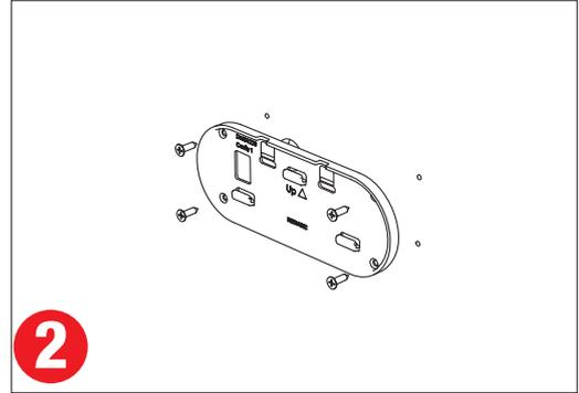
**2** Attach the Back Plate to the wall using 4 suitably sized countersunk screws.
