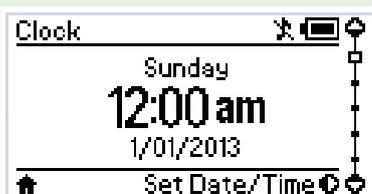
The final step required for initial setup is selecting the Time and Date to be displayed on Remote Monitor. Time and Date settings are used not only for the clock screen but also on the Charge per Hour and Charge per Day log screens. The Time and Date settings are not retained in memory so in the event that the charger loses ALL power sources (Input and Output), upon reconnection the unit will prompt the user to enter the Time and Date again.
