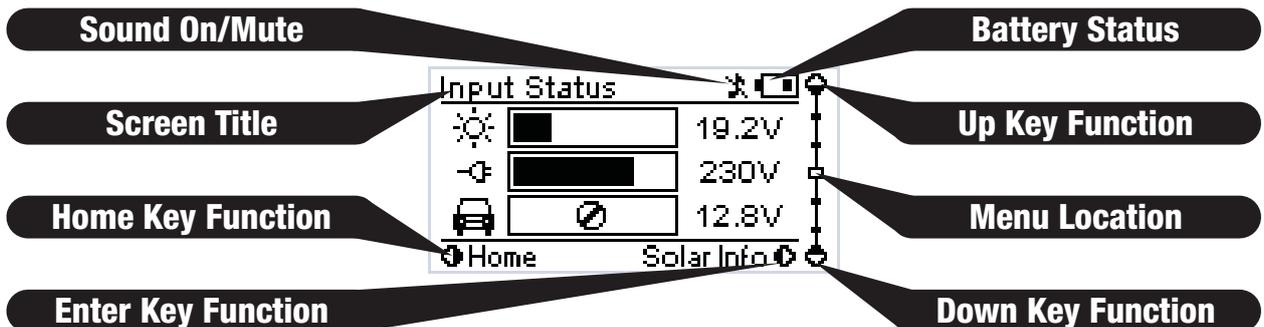
Figure 3.2.1 - The LCD Display
