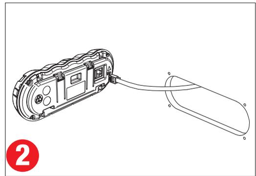
**2** Feed the Remote Monitor cable through the hole and connect it to the Remote Monitor.
