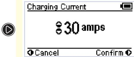
If the Charging Current setting is set lower than 30 Amps the excess current will be used to supply the loads running from the battery under charge.
