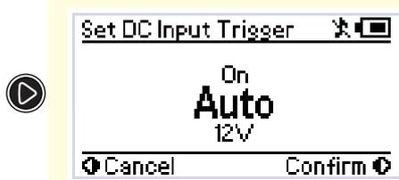
Ignition selects Ignition Trigger, Auto is controlled by The Manager30, and 12V or 24V lock the unit to a 12V or 24V system. ON means the unit can trigger DC charging whenever there is a voltage between 9 - 32V on the DC Input wire. The default value is 'Auto'.
