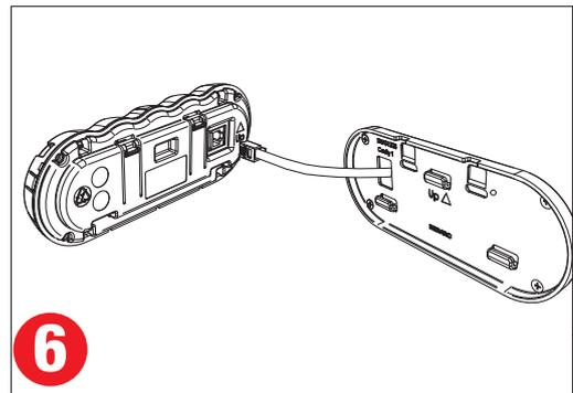
**6** Remove the Remote Monitor cable and the Inner Assembly is removed.
