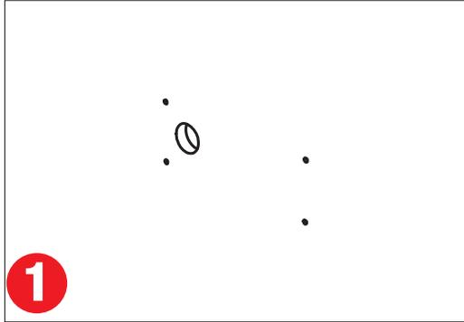
**1** Use the template provided (Page 36) to mark the position and drill and cut the mounting holes into the wall.
