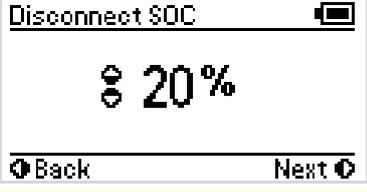
If either Voltage or SOC are selected at the Disconnect Trigger setting screen the Disconnect trigger level will need to be selected. Once the Disconnect trigger level is selected the Reconnect trigger level must be selected. Note that there is a built in minimum hysteresis constraint on this setting and a non-adjustable time delay exists to stop repetitive switching.
