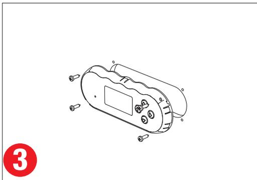
**3** Mount the Inner Assembly to the wall using 4 suitably sized screws.
