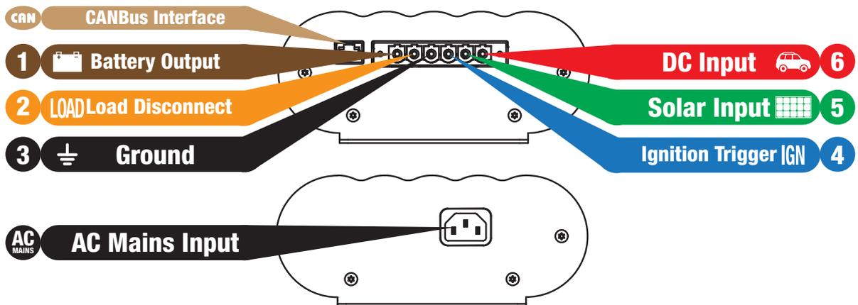
Figure 2.4.1 - Required connections.
