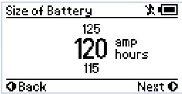
The Size of Battery screen allows the user to indicate the battery bank size. When you have chosen this value, the menu will ask for confirmation of the settings while displaying them on the screen. Refer section 2.5 for battery size calculation.
