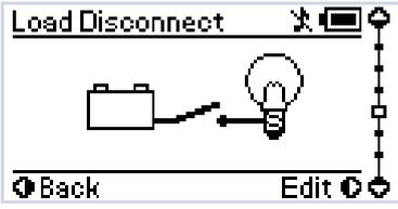
The Load Disconnect setting will output a GROUND relay trigger signal based on a user set SOC or voltage level.
