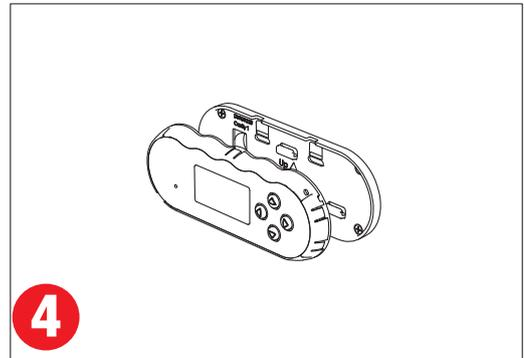
**4** Clip the Inner Assembly into the Back Plate.
