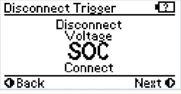
The Disconnect Trigger setting can be set to Disconnect (Loads OFF), Connect (Loads ON) or to operate from either SOC or Voltage level triggers.
