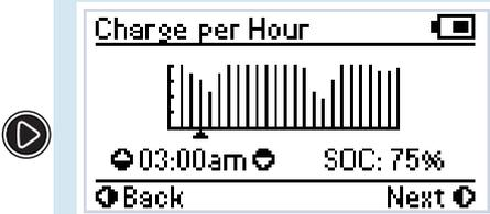
The Charge per Hour screen displays the average State of Charge of the battery under charge at the end of each hour across the course of the last day. The most recent hour is always the right most line on the graph.
