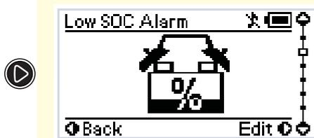
The Low SOC Alarm setting will sound an alarm when the battery State-of-Charge reaches a particular setting.
