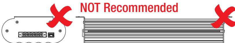
Figure 2.2.1.3 - Do NOT mount the unit upside down
