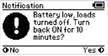
Should the Load Disconnect feature be triggered the Remote Monitor will prompt the user to allow the Loads to be reconnected for 10 minutes. This allows the user to temporarily use power (for loads such as lighting) to rectify any issues and/or engage another charging source. After this time has lapsed the load will disconnect and the prompt will reappear, unless the battery voltage is above the Disconnect level.
