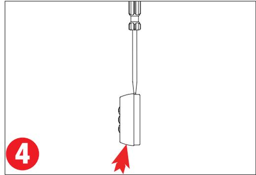
**4** When the screwdriver is in a vertical position, gently push upwards on the bottom of the Remote Assembly to unlock tab. Repeat 3 & 4 for 2<sup>nd</sup> tab.
