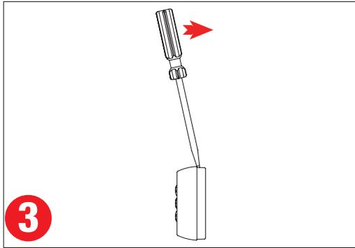
**3** Insert a flat-head screwdriver at a slight angle towards the front of the Remote Monitor and push back to depress the locking tabs.
