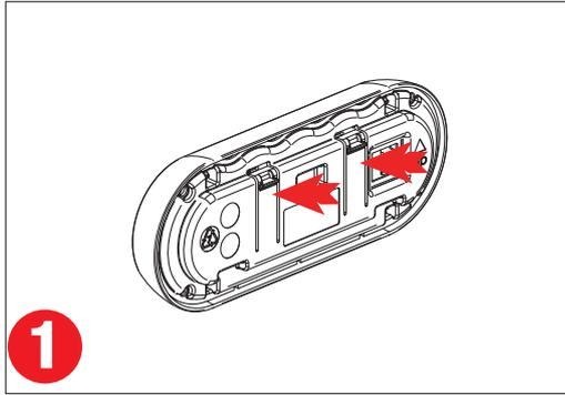
**1** The locking tabs on the back of the Inner Assembly need to be unclipped from the Back Plate.
