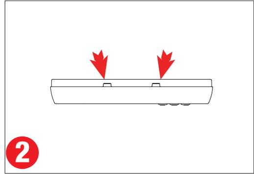
**2** The locking tabs can be accessed through holes on the top of the backing plate when installed.
