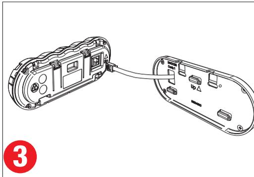
**3** Feed the Remote Monitor cable through the hole and connect it to the Remote Monitor.
