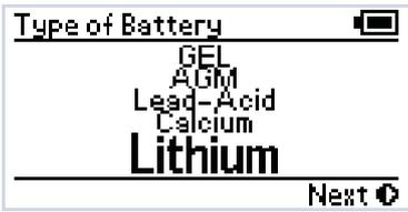
The Type of Battery screen allows the user to indicate the type of battery being charged by The Manager30. This setting will affect the charge profile that The Manager30 uses to charge the battery so it is important to select the correct battery type. Once you are happy with your selection move on to the Size of Battery screen.
