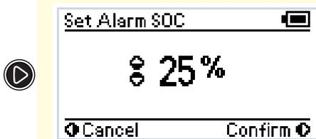
The Set Alarm SOC setting sets the percentage of State-of-Charge at which the alarm will sound. The Alarm SOC can be set to from 0 - 100%.
