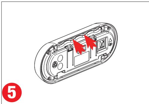
**5** Slide fingers between the Front Face and the Inner Assembly in positions marked above and carefully pull back towards the front of the Remote Monitor.
