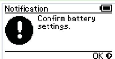
The second and most important step required for initial setup is Battery Type and Size selection. Please refer to the battery manufacturers specification sheet for Size(AH) and Type specifications. If you are unsure of the type of your battery please select the Gel setting. Should power to the Battery Sensor be removed at any time, the unit will revert to the Gel setting and prompt the user to input their Battery Type again. The Battery Size setting will be retained in memory.
