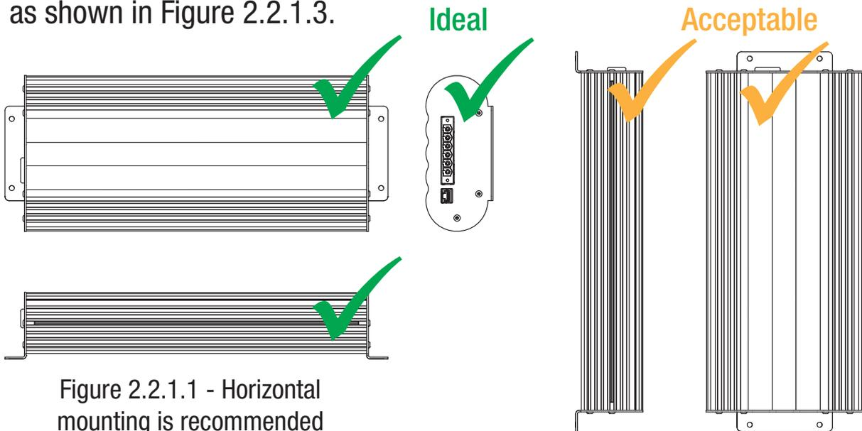
Figure 2.2.1.1 - Horizontal mounting is recommended
