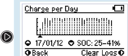
The Charge per Day screen displays the maximum and minimum State of Charge of the battery under charge for each day across the course of the last month. The most recent day is always right most line on the graph.
