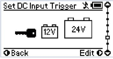
The DC Input Trigger allows you to select whether you would like your DC input to be triggered via Ignition, automatically via The Manager30, or at a specific voltage.
