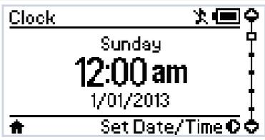
The Manager30 features a real time clock (time and date) function which needs to be setup when the power is first connected.
