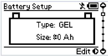
The first screen in the Settings menu is the Battery Setup screen. The Battery Setup displays the selected battery settings for the battery under charge.
