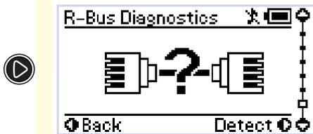
This screen is used by REDARC to identify problems with a The Manager30 setup and does not need to be accessed unless requested by REDARC Technicians.
