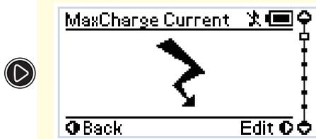
The MaxCharge Current setting refers to the amount of current permitted by The Manager30 to charge the battery, up to a maximum of 30 Amps.
