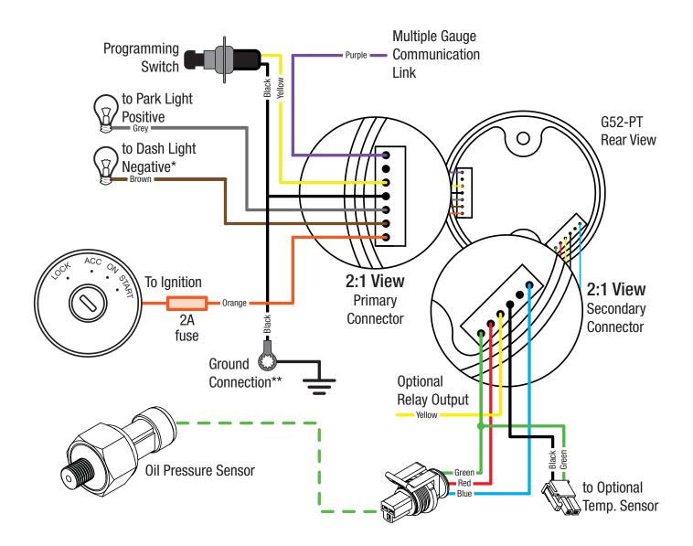
\* Connect to a dash light that dims via the vehicle dimmer adjustment to ensure the gauge dims accordingly. If your illumination circuit in your vehicle varies the positive voltage for dimming you will require an Redarc Enhanced Lighting Controller (GA-ELC) to get the gauge to dim with your night-time driving light.
