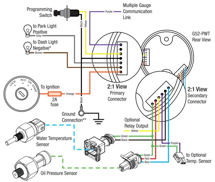
\* Connect to a dash light that dims via the vehicle dimmer adjustment to ensure the gauge dims accordingly. If your illumination circuit in your vehicle varies the positive voltage for dimming you will require an REDARC Enhanced Lighting Controller (GA-ELC) to get the gauge to dim with your night-time driving lights.
