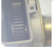
Now insert the drum retention plate. Please take care that the plate locates in the correct groove as shown opposite.
