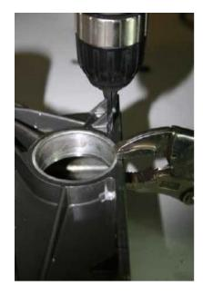
Once the shim is positioned, secure using a suitable clamping device (e.g. mole grips)
