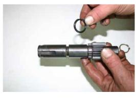
Remove drum from lower housing and clean all parts thoroughly. The original main shaft can now be discarded.
