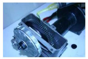
Now refill the lower casing with 0.2 litres of EP 80/90 or 30 SAE oil
