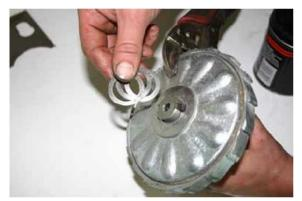
Now fit to brake to the main shaft. Do not forget to refit the woodruff keys and shims if the original winch had them fitted
