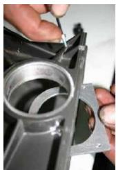
Refit drum and large gear to lower casing, and locate modified retention plate inside casing.
