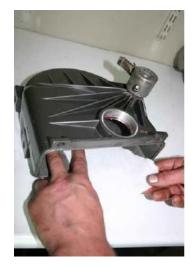
Take the now clean lower housing and place a cloth or rag to protect the bearing as shown.
