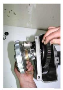
Holding the brake assembly using the mole grips, remove the circlip from the end of the shaft. Remove the brake from the shaft and place in a safe place.
