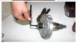
Using the template supplied, modify the shaft retention plate to allow the newmain shaft to fit.
