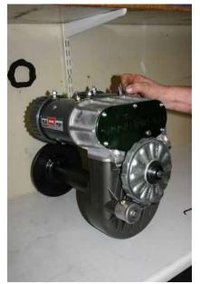
Your winch is now ready to be installed into your vehicle. Please ensure that the breather is routed to a high point on the vehicle were water and dirt ingress are unlikely.
