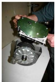
Apply a bead of silicone type sealant to the top housing and fit to the winch taking care that correct location and meshing is achieved.
