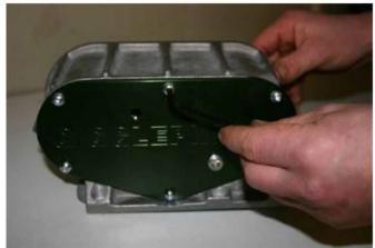
Without using sealant fit the new top housing to the winch taking care that it locates correctly.
