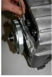
Using the scribe, mark the position of the new mounting on the lower housing, using the top housing as a guide.
