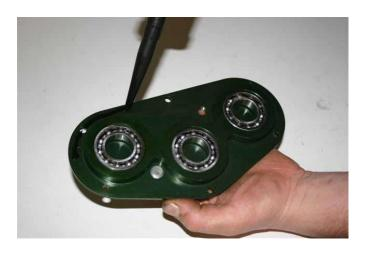
Before fitting the bolts take care that the special washers are fitted correctly with the raised inner facing the bolt head.
