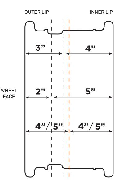
UTV Offsets are represented in an equation such as 4+3 or 5+2. The first number indicates the distance from the inner lip to the mounting surface. The second number is the distance from the mounting surface to the wheel's outer lip
