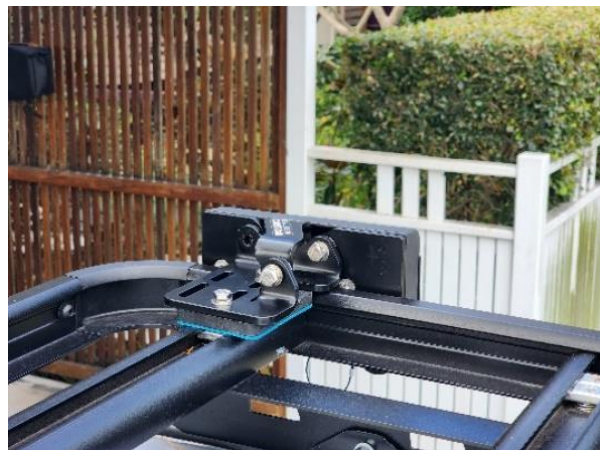
*XD Side Twist Short Foot Bracket on Platform Style Transverse Bars/Slats * Wedgetail Platform Rack shown with packers under bracket foot
