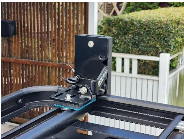
*XD Side Twist Short Foot Bracket on Platform Style Transverse Bars/Slats * Wedgetail Platform Rack shown with packers under bracket foot
