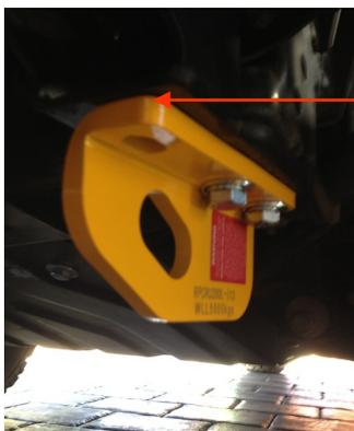
Additional BOLT (not supplied) to be positioned here (most forward mount hole) where paired with a TJM & Ironman bull bar.
