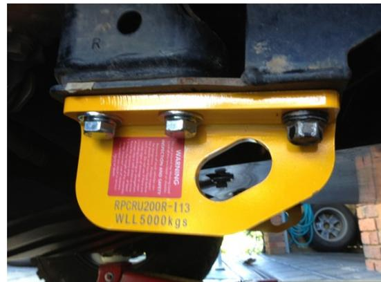
**Ensure all supplied and specified components are used during the installation of tow recovery points, Failure to do so will significantly reduce the Working Load Limit (WLL) specified for each individual point (5000kgs for 200 Series Cruiser), which can result in serious injury or death.**
