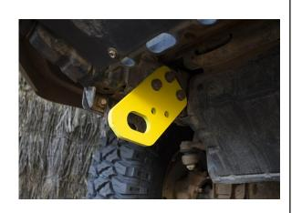
Although RP-PAT01 is supplied individually—it is recommended that any pull applied to the tow point is done so using a corresponding attachment point to the chassis on the other side of the vehicle, so as to evenly distribute the force across the two tow points.
