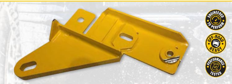
Applicable to vehicles manufactured post JUNE 2018. A stiffening plate installed inside the chassis rail affects access to one hole used in the fitment of RP-RAN02 (Refer Image). Using a step drill enlarge this hole to allow fitment of the supplied hardware. The spacer pictured will require modification to clear the new weld not present on previous vehicles. The nut plate will sit behind the stiffening plate, with the bolt passing through.
