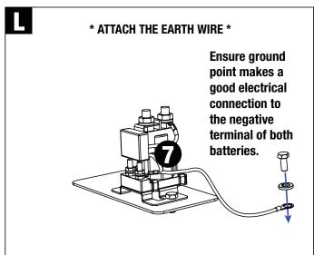
Wire the SBI12 as shown in diagrams M,N & O. Ensure that all connections are tight and that the provided spring washers are used.
