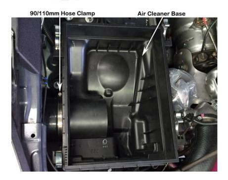
Align the air entry hose for best fitment (Ensure the air entry hose is installed hard up against the shoulder of the snorkel body outlet), correctly position the 90/110mm hose clamps at either end of the air entry hose and tighten the hose clamps.
