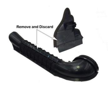
Remove and discard the perforated section from the guard panel template (item 13) as shown.
