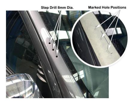
Install the plastic inserts (Item 6) into the 8mm diameter holes in the A-pillar.
