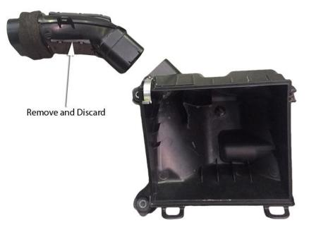
Remove and discard the air intake duct from the air cleaner base.
