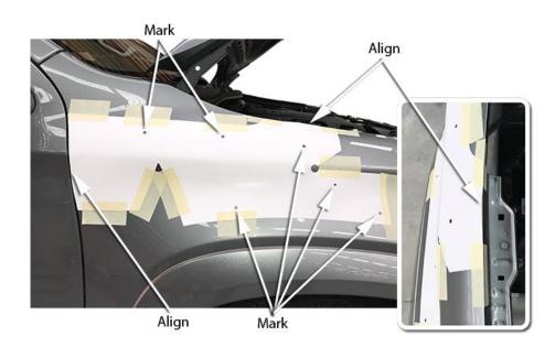
Drill a pilot hole for each of the marked hole positions.
