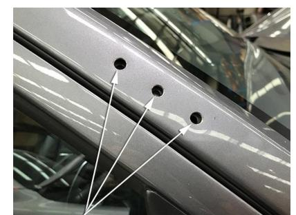
Drill A-pillar Panel 8mm, Inner Panel 6mm
