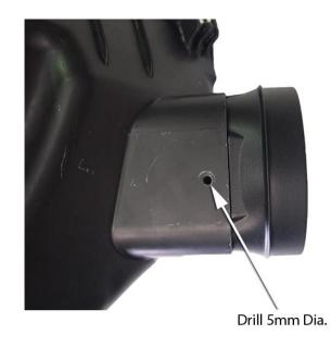
Apply adhesive sealant to the inside of the air cleaner base inlet and the outside of the air cleaner inlet adaptor (item 10).
