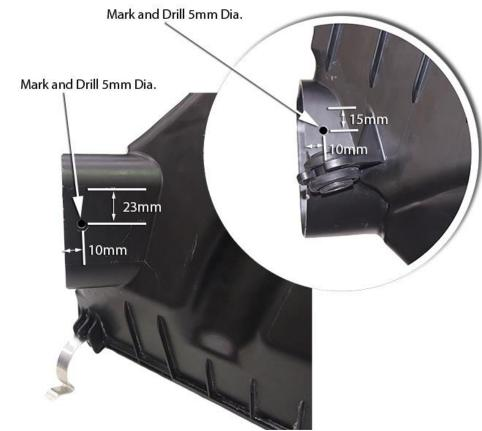
Measure and mark two hole positions on the air cleaner base inlet approximately 10mm in from the end of the air cleaner base inlet and 23mm (long side) and 15mm (short side) down from the radius of the inlet as shown.
