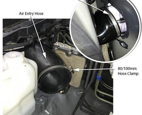
Re-install the air cleaner base, guiding the air cleaner inlet adaptor into the air entry hose, fasten the air cleaner housing using standard
