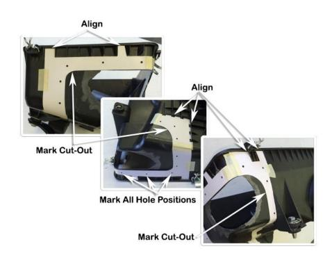
Using the body saw cut the new air cleaner base inlet hole as marked in step 14, using the body saw remove the two internal ribs shown.
