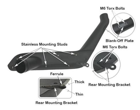
Apply loctite 243 to the remaining two M6 x 12mm Torx bolts (item 10) and secure the rear mounting bracket (item 8) to the snorkel body as shown.
