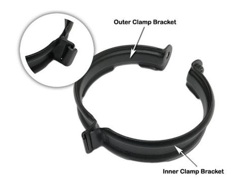
Install the outer and inner clamp brackets (item's 4 & 5) around the air ram, ensure the brackets are positioned over the 4 upper moulded lugs on the air ram.
