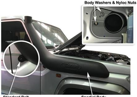
Install the rubber bracket gasket (item 6) to main upper mounting bracket (item 3), using the 2 x M8 A-pillar bracket genuine bolts retained in step 2, secure the main upper mounting bracket with rubber gasket installed to the 2 captive nuts in the A-pillar.
