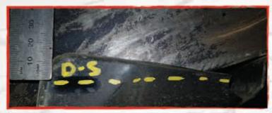
Picture above is of the drivers side front bash plate, similar amount needs to be trimmed, again placing the bash plate back into position will show how much of this wing that needs to be trimmed. Paint cut surface to stop rust forming.
