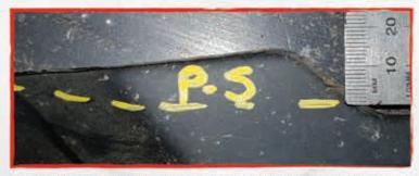
Picture above illustrates trimming required of the passenger side factory bash plate. Self explanatory once the recovery points are fitted and the bash plate sat in position.
