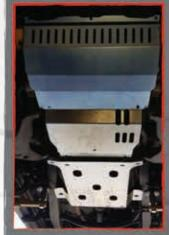
These two pictures are fitment of the RPTRI02 with Roadsafe under body protection. No modification is necessary.
