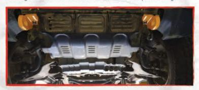
For fitment with factory bash plates ensure that there is 6mm or more clearance around the recovery point allowing for chassis deflection.
