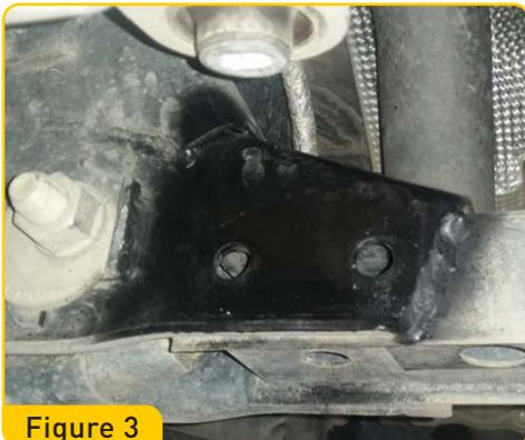
4. Fit bracket as shown in images using the 2 x M10x1.50P x 110mm long bolts with M10 flange nuts and washers supplied. Reinstall factory bolt through diff mount into new bracket. Fit supplied washer and flange nut; leave loose until the end of installation procedure. See figures 4 & 5.
