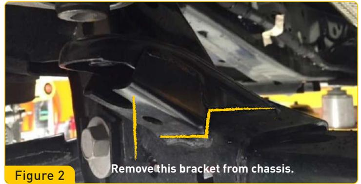
3. Once removed, clean the area with a flap disc and paint to avoid future corrosion. See figure 3.
