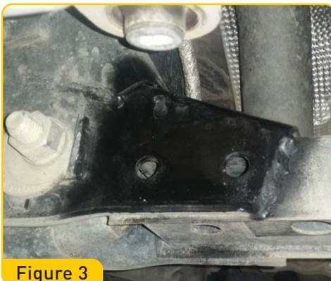
4. Fit bracket as shown in images using the 2 x M10x1.50P x 110mm long bolts with M10 flange nuts and washers supplied. Reinstall factory bolt through diff mount into new bracket. Fit supplied washer and flange nut; leave loose until the end of installation procedure. See figures 4 & 5.
