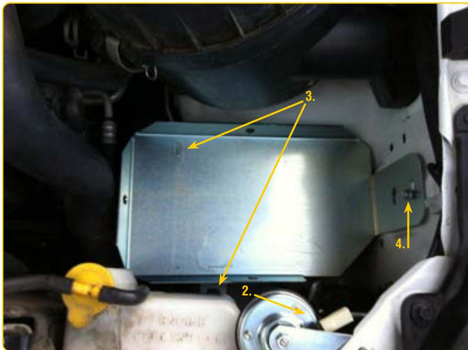
3. The tray has two support brackets under it. For the support towards the engine, use the existing bolt. The second support is to the front of the vehicle; use 6mm bolt, washers & nut.
