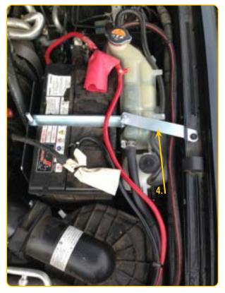
Once the battery has been placed in the tray, hold down fitted there is a support bracket bolts to the guard and fixes to the hold down bracket.
