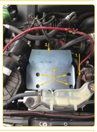
3. The tray also has a heat shield that bolts to the tray using 4mm bolts & nuts after the tray base, is in position and all bolts are tighten.
