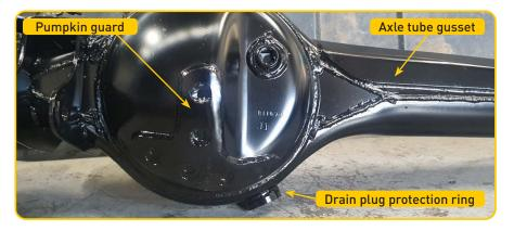
7. Mount housing on a support structure. This structure and the method of mounting need to be rigid enough to resist any distortion in the housing due to welding.
