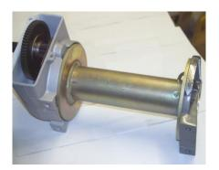
Before fitting the winch to the vehicle, please check that your winch mount/plate is straight and square. This is very important. If your mount is bent or buckled it will need replacing before the free spool will operate correctly.
