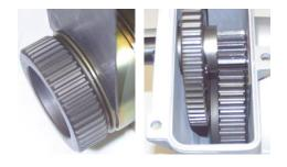
Now insert the drum retention plate. Please take care that the plate locates in the correct groove as shown opposite.
