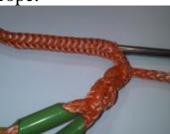
Step 7: Ease the fid out through the side of the rope (Pic a), remove it from the rope, and remove any electrical tape from the rope (pic b)
