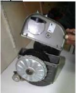
Using the 1/4" Alley key, remove the 3 bolts that secure the upper motor housing & place to one side.
