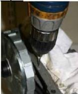
With the centre punch spot, mark the centre of the scribe mark. Then make sure to protect the inside from swarf.
