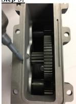
Apply a bead of silicone type sealant to the top housing groove and fit the winch taking care to ensure the correct location and meshing is achieved.
