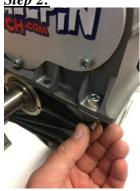
Without using sealant fit the new top housing to the winch taking care to make sure it locates correctly.
