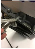
Using a scribe, mark the position of the hole behind the brake assembly new mounting on the lower housing, using the top housing as a guide.
