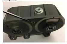
The 1/8 BSP blanking plug can be removed from between the motor mountings and a breather pipe installed – optional kit available. G17012 – GP Pro Winch Breather Kit.
