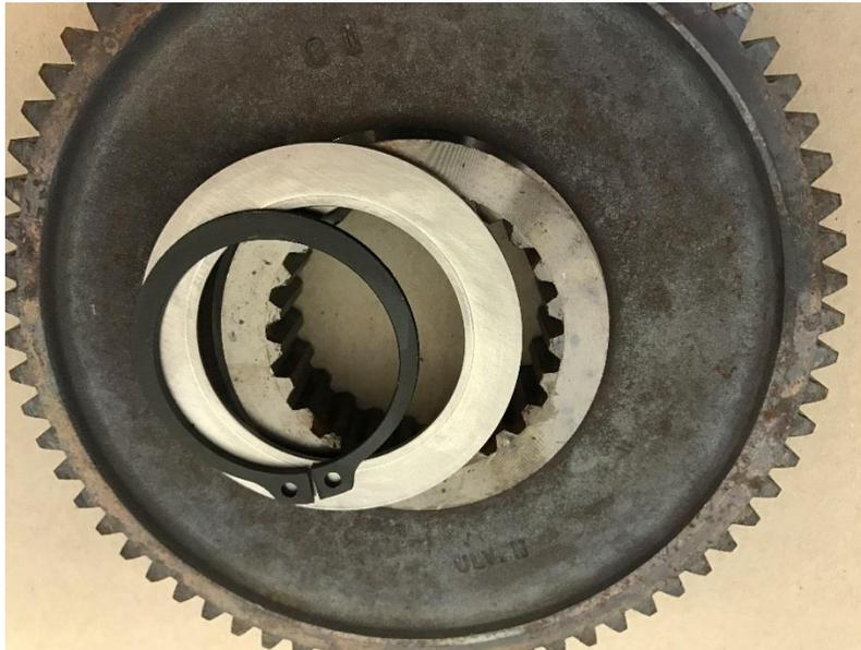
Now slide the large cam gear over the mainshaft and insert the mainshaft, taking care to fit the large intermediate gear, round shim and circlip.
