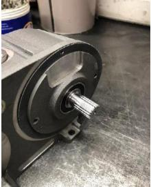
Slide the gear shaft onto the installed drive shaft, with the gear teeth closest to the top housing.
