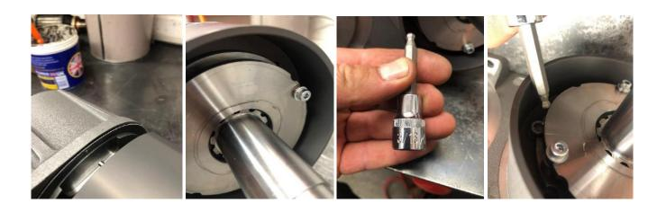
The next step is to install the end cap, with the air fitting on the top, fit the 4 x M6 cap head bolts and schnoor washers, using a little copper slip on the threads, tighten with a 5mm allen key.
