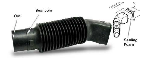
Place a 70/90mm hose clamp (Item 11) over the other end of the cuffed hose (Item 10) and install the cuffed hose to the modified plastic connection duct.
