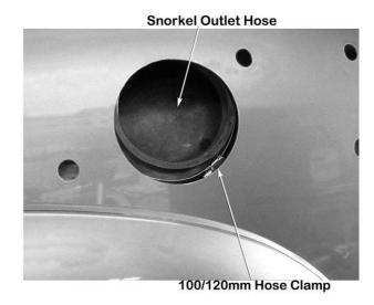
12 Carefully install the snorkel body (item 1) to the guard panel guiding the snorkel body outlet snout into the snorkel outlet hose (item 10), align the snorkel body to the guard panel and upper mounting bracket. When correctly aligned fasten the snorkel body to the guard panel with body washers (item 8) and nyloc nuts (item 9). Fasten the snorkel body
