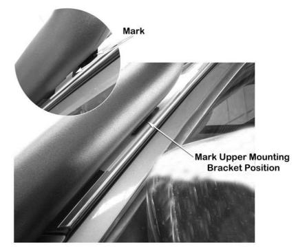
Remove the snorkel body (item 1) from the vehicle and remove the upper mounting bracket (item 3) from the snorkel body.
