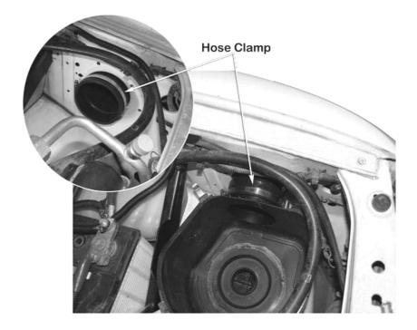
Align the two hoses (items 10 &12) for best fitment, ensure that the snorkel outlet hose (item 10) is installed hard up against the shoulder of the snorkel body outlet snout, tighten the 100/120mm hose clamp (item 15).
