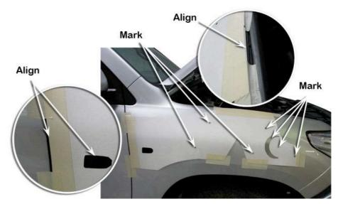
Drill a pilot hole for each of the marked positions.
