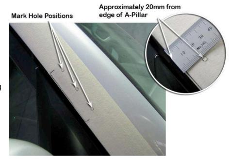
Drill a pilot hole for each of the 3 marked hole positions on the A-Pillar.
