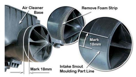
12 Install the air entry hose (Item 14) onto the air cleaner inlet snout and align the moulded part line of the air entry hose to the marked position on the air cleaner inlet snout as shown.
