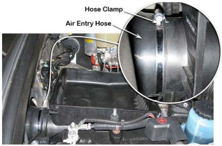
Loosely install a 90/110mm stainless steel hose clamp (Item 15) onto the snorkel snout end of the air entry hose (Item 14) and ensure that the clamping bolt of the hose clamp is orientated for accessibility.
