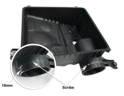
Using a scribe or paint pen, scribe or mark a line 18mm in from the end of the air cleaner inlet snout around the entire circumference as shown.
