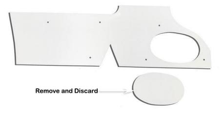
Align the guard panel template (Item 16) to the upper and rear edges of the right hand guard panel as shown.
