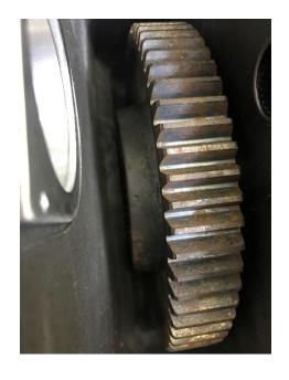
Now slide the two cam gears over the mainshaft (fitting the O Ring first) and insert the mainshaft, taking care to fit the large intermediate gear, round shim and circlip.
