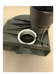
Fit the shim to the inside of the casing, ensuring that it is aligned with the mainshaft aperture and that the top of the shim does not protrude past the edge of the casing.
