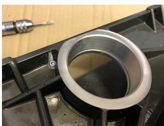
Before fitting the shim to the casing, use a 3.5mm drill bit to widen the holes in the casing.
